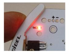
Depress the whiskers, the LEDs are lit when the corresponding microswitch is on.
