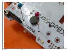
Turn upside down and insert 2 positionning pins
