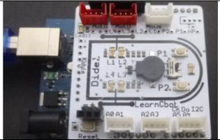
No motor, but bicolor leds tho show the speed and direction of motor. No whiskers, but 2 push button. So much to learn and experiment before investing in a robot.
