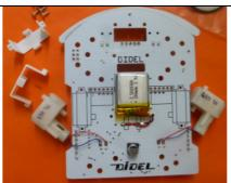
Prepare the brakets that hold the motor.
