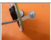
Turn not loosing the screw and position the caster.
