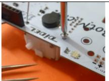
Screw, but not fully, wait for the seond srew in place. Do not force. Check for alignment.
