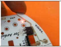
Power on. If the twin LEDs are not on, it's time to charge. Check the whisker's LED..
