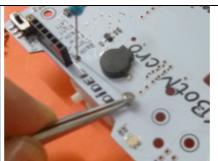
Center as well as possible Depress on the card and position the screw.
