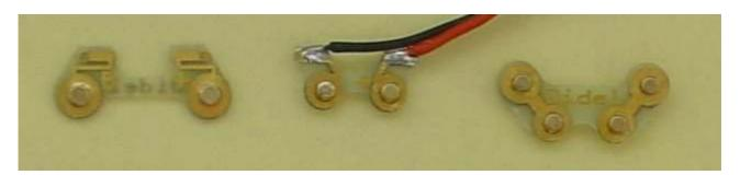
The Bapi/Bami circuits have two tabs on solder can be applied connection to the battery tabs or the wires toward the receiver. When soldering, the heat must not travel toward the magnet. The Bapi-B (on the battery side) and the Bapi-M (on the model side) are not identical due to magnet orientation, like male and female power plugs.
