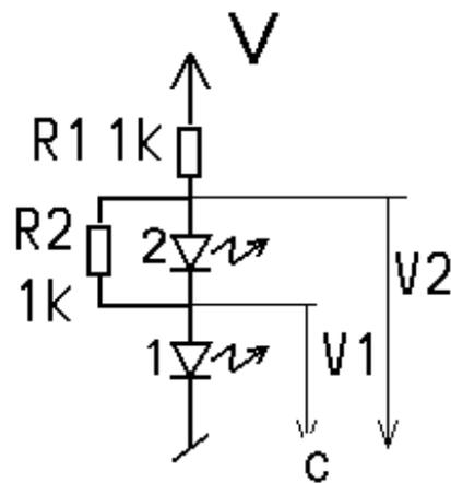
Let us assume that we use red LEDs that start to light at 1.8V, and then have an internal resistance we can assume to be very small, so the voltage of 1.8V will not change significantly.
