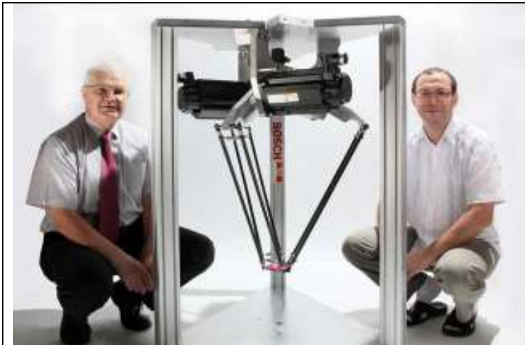
The Delta robot, invented by prof Clavel at the EPFL, Switzerland, is cute and fast.
