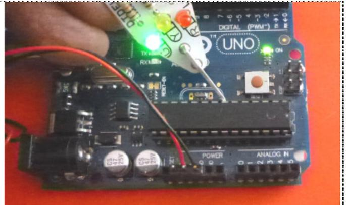
Note: you have to power from the circuit you test, or have a common ground
