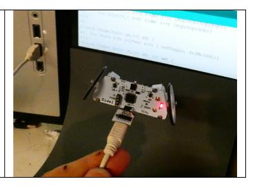
The card is indeed an Arduino AVR328 compatible board with an external serial to USB module.
