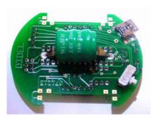
Solder the resistance and capacitor first. Fold the wires, solder, check, cut.
