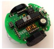
The kit consist of 3 PCB, 2 motors with wheels, 1 NiCd battery 3.6V 100 mAh, socket for processor with pin-out compatible with 16F870, RS232, buzzer, programming and extension connector.
