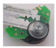
Position the motor PCBs. Solder at one point, check for perpendicularity. When perfectly aligned, solder all points both side.
