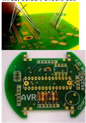
Insert all the sockets. Return on a piece of wood and solder one pin of every connector. Check for correct insertion, solder all.
