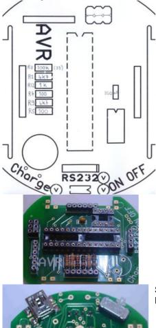
Be carefull not doing a short between USB pins. Only the side ones are soldered.
