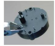
Insert the wheels. Put a piece of 0.2 to 0.4mm thick piece (thick paper, two razor blade) as a spacer
