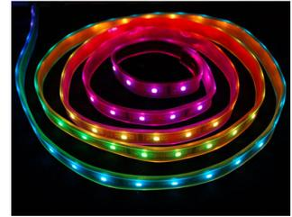
The leds of a strip are serially connected and use shift registers. As shown later, shift registers are controlled with a clock and a data line. A third information is required to know when the data is complete. SPI add a third line. RGB strips count the clocks or no clock for e.g. 10ms means the end of transmission. RGB smart leds with 2 control lines accept a clock frequency up to 20 MHz and include the early WS2801 and by 2017 the one-chip APA102C, APA102-2020 and Sk9822 listed in appendix.
