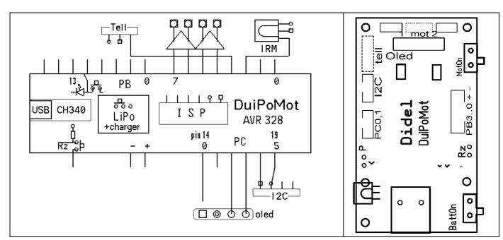
The DuiPoMot includes a AVR328, a CH340 USB controller (miniUSB plug), two CS7721 bidirectionnal motor drivers (max 0.4A) The 328 is loaded with the Duemilanove driver. There is an IR module. See the definition file and start programming, it is just an Arduino.
