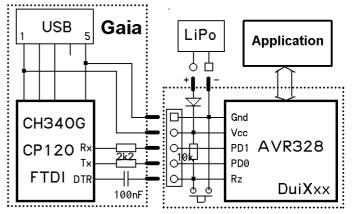
We do the same with Gaia and the Dui family. Gaia uses the easy CH30G USB driver and the pinout of the connector is well defined for 2.54mm strips and 1.27 connectors. Gaia always has a male connector. Dui boards do not have a connector, just the holes in which Gaia pins are inserted and maintained in such a way the good contacts are guarantied for the short duration of programming. When soft development is made on a board, a female connector is soldered.
