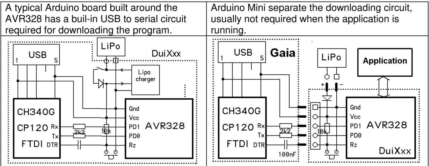
We do the same with Gaia and the Dui family. Gaia uses the easy CH30G USB driver and the pinout of the connector is well defined for 2.54mm strips and 1.27 connectors. Gaia always has a male connector. Dui boards do not have a connector, just the holes in which Gaia pins are inserted and maintained in such a way the good contacts are guaranteed for the short duration of programming. When soft development is made on a board, a female connector is soldered.
