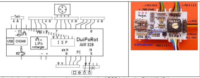
A typical application is to control a wearable strip of RGB leds or the Didel MiniCube.
