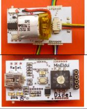
The DuiPo is compatible Arduino Duemilanove and include on request a 200mAh LiPo. Any Lipo is easy to solder.
