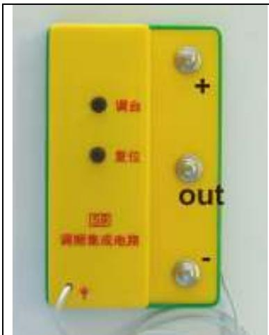
The **FM Module** (not in SC-100 or SC-300) contains an integrated FM radio circuit. The inside looks like this:
