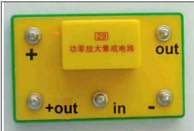
The **power amplifier IC module** (not included in model SC-100) contains an LM386 audio amplifier IC and supporting components. Its actual schematic looks like this:
