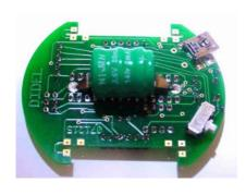
Solder the battery. Note on this proto serie the pads does not correspond. Bend the battery leafs a maximum.
