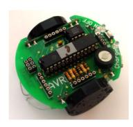
The kit consist of 3 PCB, 2 motors with wheels, 1 NiCd battery 3.6V 100 mAh, socket for processor with pin-out compatible with 16F870, RS232, buzzer, programming and extension connector.
