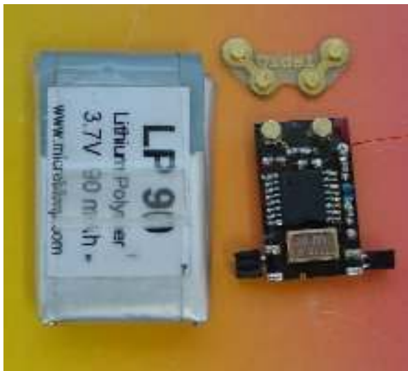
90 mAh and 20 mAh Lipo on a 2 channel Butterfly receiver.
