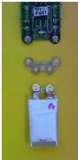
30 mAh Lipo with 5mm Bahoma (Bami) on a Md41 Didel IR receiver. Bada on Tricha
