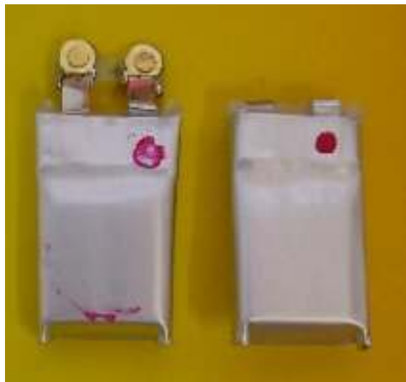
Bamis soldered to a 30 mAh ABF lipo
