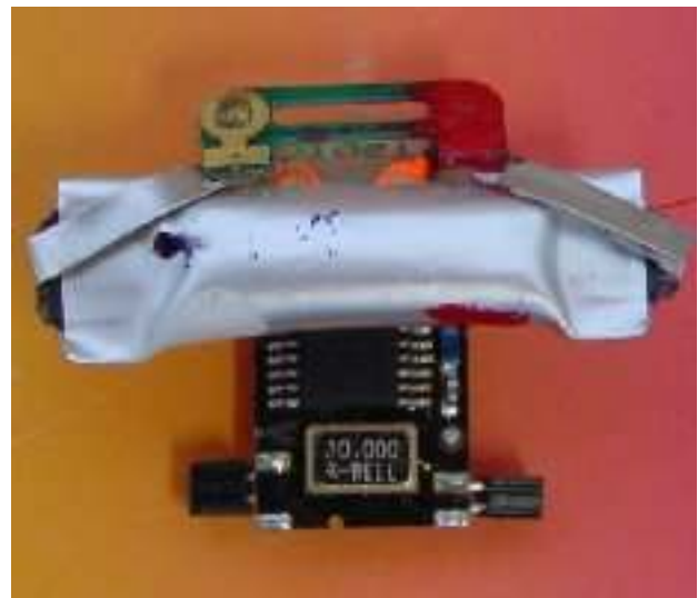
90 mAh and 20 mAh Lipo on a 2 channel Butterfly receiver.
