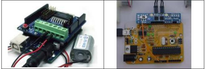
Let's have a motor or bicolor Led connected to pins 4 and 5. Pin 4 is set a LOW and pin 5 receive an 8-bit PWM value. (analogWrite(value). Now if one wish to reverse the rotation, one need to put a HIGH on pin 4 and set the PWM value on pin 5 to be the complement of what we need. That is, if one need a low speed, a high "analog" value is required, so the difference with the HIGH of the other pin is small. The complement, 255-value, must be used as shown in next picture.
