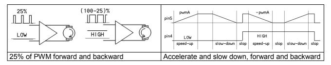
You have a robot with two motors? Undersand how to control the motors with digitalWrite (on all pins) and then with analogWrite (only on pins 5 and 6). Wire you motors so that you define
