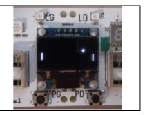
The racket is 16 pixels high and its high point moves from 0 to 48. The formula (3x (256-Pot) / 16 gives a value from 0 to 48 with the value 0 when the pot is at the top.
