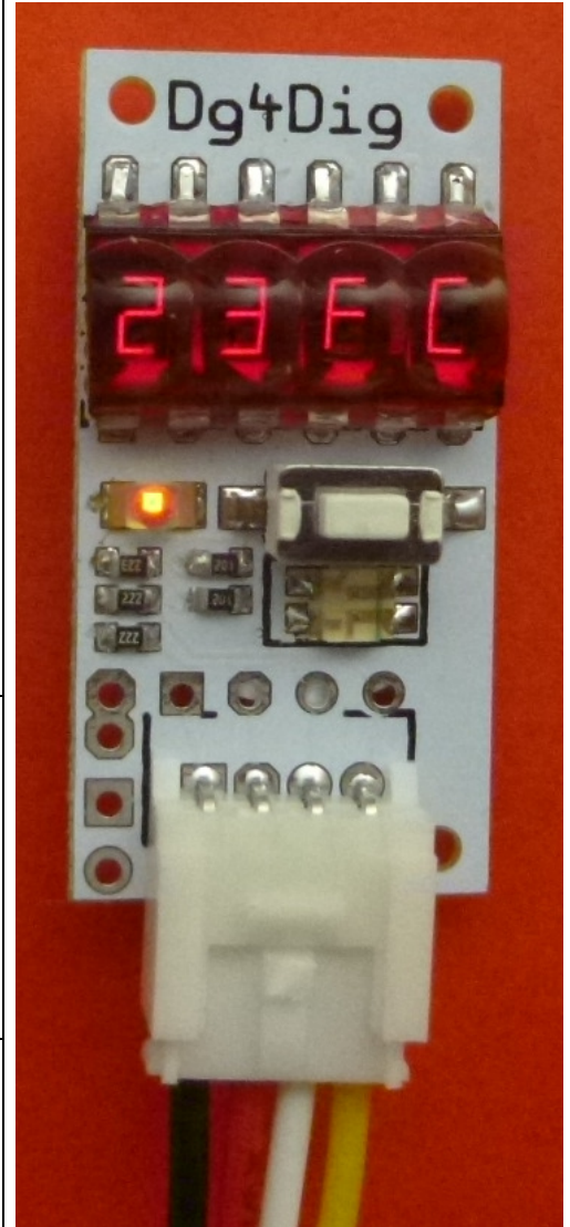
Grove connector pinout: Gnd Vcc SDA SCL
