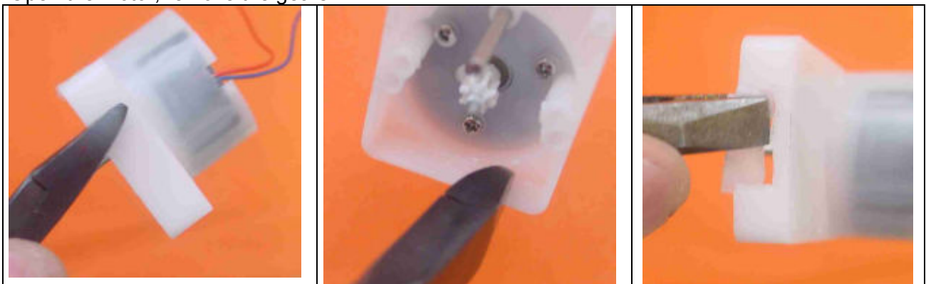
Use a plier cutter and a plier to cut an break the side next to the motor, leaving 4-5mm every side
