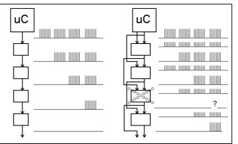
Before that, the WS2813 which is one-wire and does not need to use next trick, solves partly the reliability problem.
