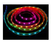
The leds of a strip are serially connected and use shift registers. As shown later, shift registers are controlled with a clock and a data line. A third information is required to know when the data is complete. SPI add a third line. RGB strips count the clocks or no clock for e.g. 10ms means the end of transmission. RGB smart leds with 2 control lines accept a clock frequency up to 20 MHz and include the early WS2801 and by 2017 the one-chip APA102C, APA102-2020 and Sk9822 listed in appendix.
