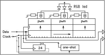
As said before, each circuit takes the first set of clocks and data he receives for himself, not transmitting that information further. The next clocks and data are amplified and transmitted. The delay introduced between each LED may be noticed over very long strips.
