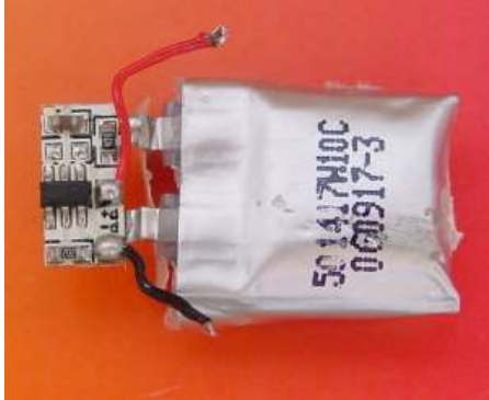
Taking out the PiccoZ Lipo circuit to build an adapter for any Lipo (uses a Bami-B)
