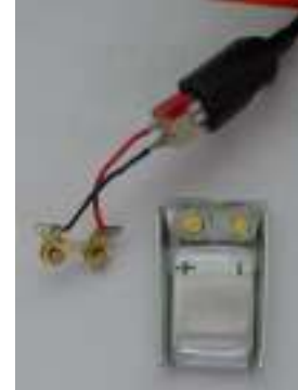
Lipo adapter for a PiccoZ clone (uses a Bami-M)
