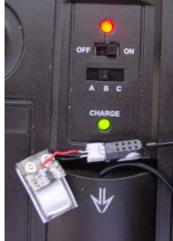
Lipo adapter for a PiccoZ clone (uses a Bami-M)
