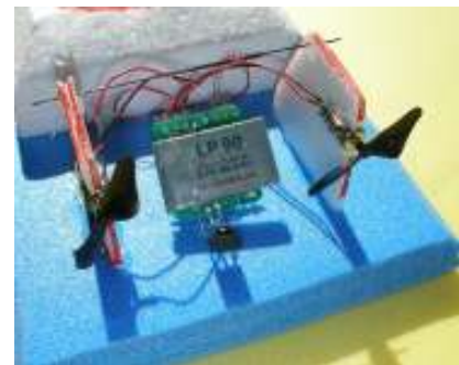
Hoovercraft model, controlled by an lbzTwin circuit (built by Urs Szymanski, Switzerland)
