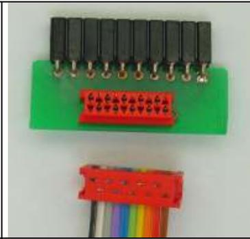
Power and 8 data lines can be transferred to some distance using a flat cable and the easy to get Micromatch connectors.
