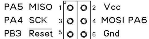
AVR programming connector for Tiny 24/44/84
