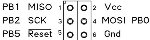
AVR programming connector for Tiny13A
