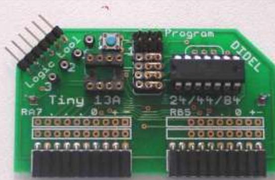
The board is designed to test the two major processors of the ATmega famils, in 28 and 40-pin DIL package. Compatibility with other 28 and 40-pins AVR processors has not been verified.
